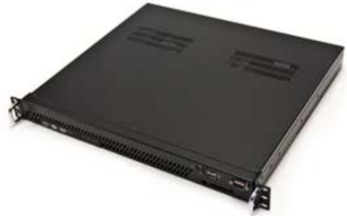
Intel Core2 Duo 3.0GHz, 2Gb RAM, 60 Gb solid-state hard drive. Certified to IEC60945. One Unit high (1.75") 19" rack-mount case with brackets. Measures 433 x 390 x 45mm excluding brackets. Weight 6.8 Kg.
