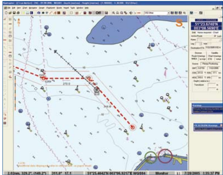
Vessel underway with heading marker set to show predicted position at user-defined intervals.
